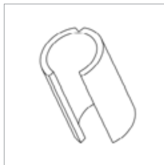
Adapter \varnothing 30 for tube \varnothing 38
